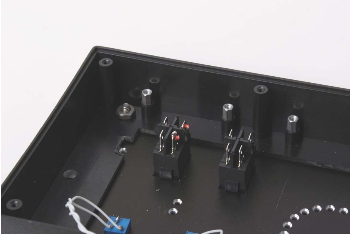
Upper Enclosure Piece with 6-32 x 0.250" stand-offs installed
