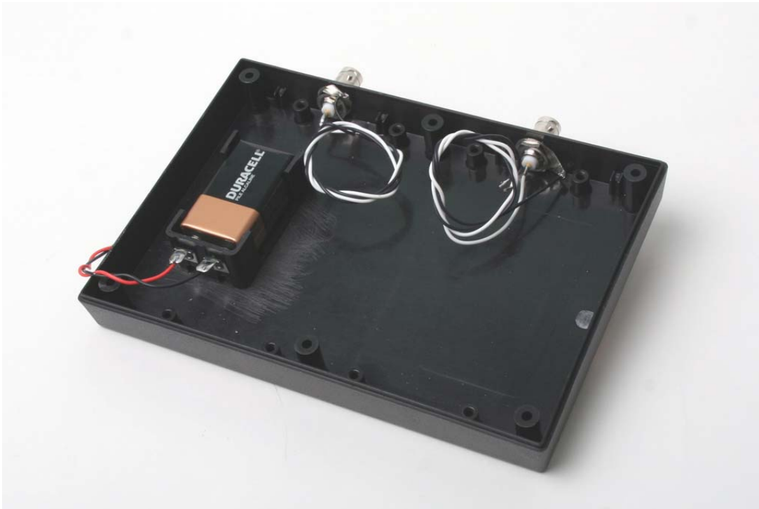
Bottom Enclosure with 9V Battery Holder / BNC Connectors
