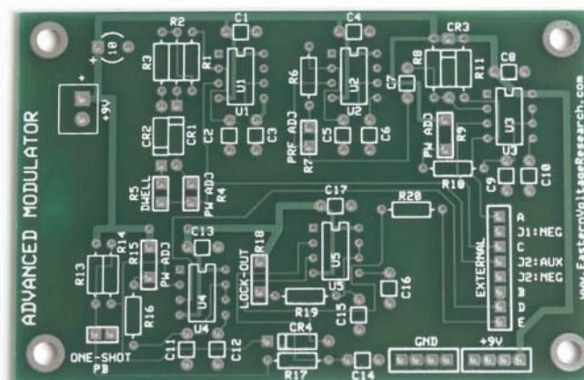
*Advanced Modulator Printed Circuit Board*
