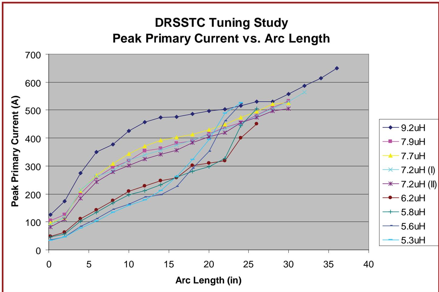
Figure 6-6 Peak Primary Current vs. Arc Length (PRF = 100Hz, Pulwidth = 300us)
