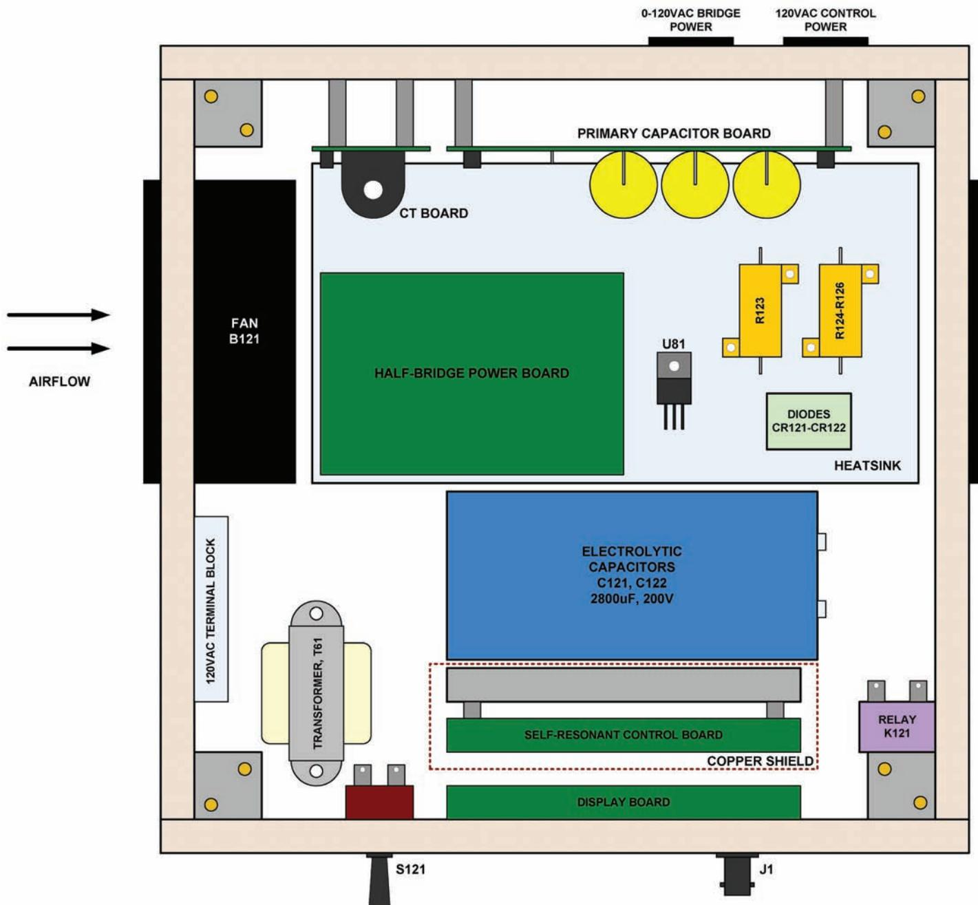
Figure 2-11 *miniBrute DRSSTC Enclosure Layout*
