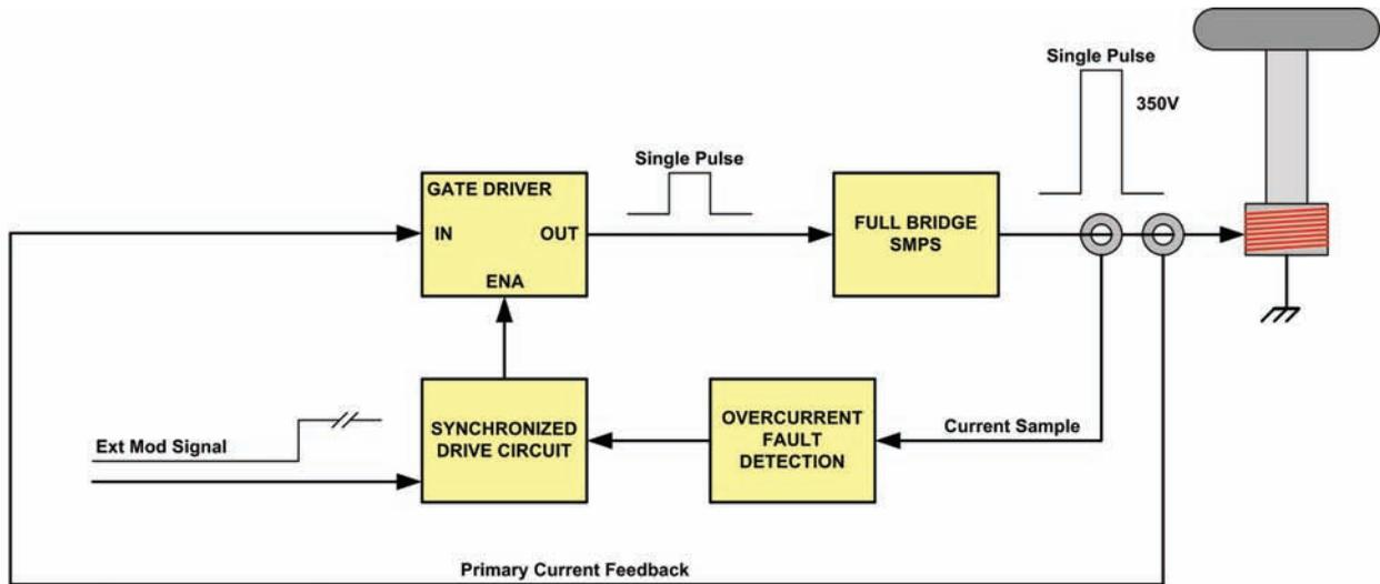
Figure 1-2 miniBrute DRSSTC Operation - Self Starting
