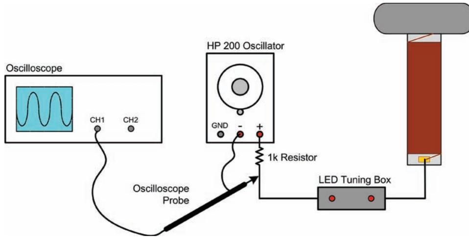
**Figure 5-8** *Secondary Coil Resonant Frequency Measurement Set-up*
