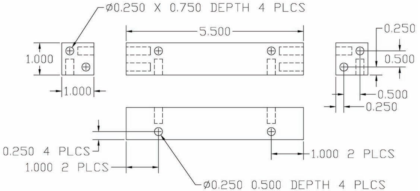
**Figure 3-3** Inner Support Detail
