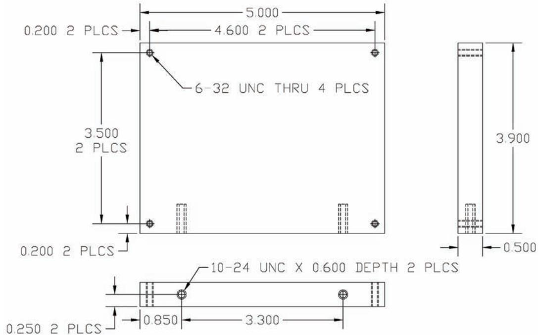
**Figure 3-8** *Self-Resonant Control Board Mounting Block*
