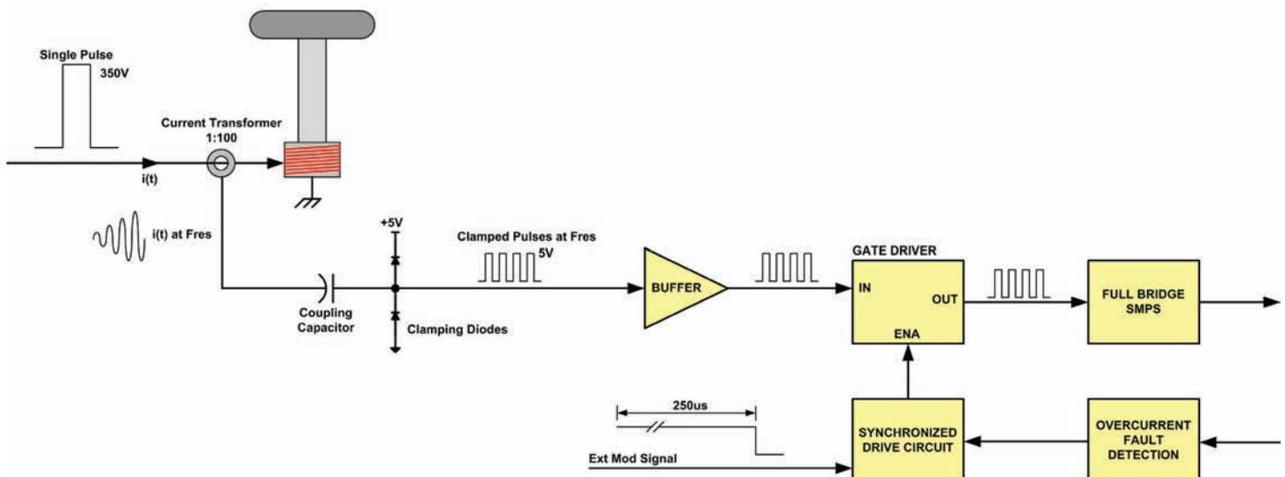
Figure 1-3 miniBrute DRSSTC Operation - Primary Current Feedback
