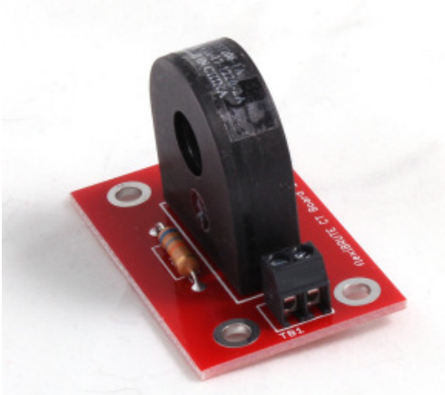
Current Transformer Board 1.0
