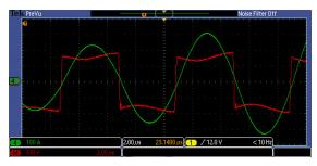
Figure 3 – Optimally Tuned DRSSTC System
