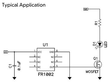
Note: A 0.1uF bypass ceramic capacitor is required.
