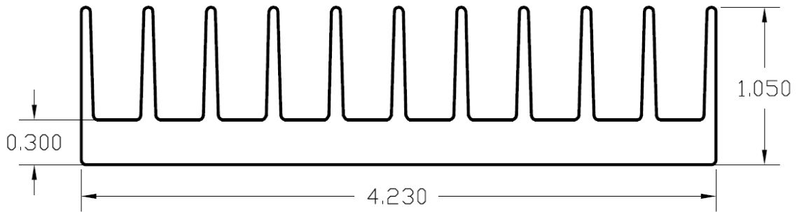
Heatsink 4.2 Profile (Thermal Impedance 2.15 °C/W/3.00")
