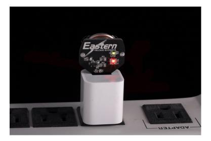
This USB powered battery charger is used to charge the LIR2450 Lithium-ion batteries used in our HP Candle Module 1.0B units. This charger is designed for both RCR2450 and LIR2450 rechargeable Lithium-ion button cell batteries and is powered directly through a USB port. Two onboard LEDs provide the user with a status of the battery charging. One LED is used to indicate the battery is charging while another LED is used to indicate the battery charge cycle is complete and ready for use.
