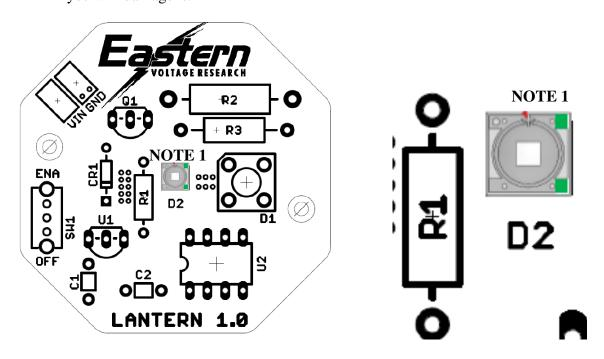
Note 1: IMPORTANT. The diagram above is incorrect. The green squares should be on the LEFT side of the component, not the right as shown above.
