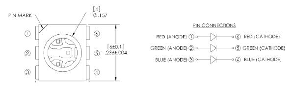
Place the LED on the board with the notch oriented toward the silkscreen DOT on the board.
