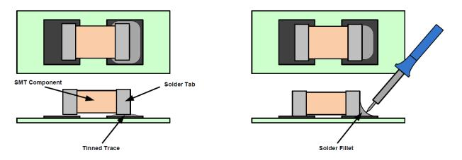
At first, surface mount soldering may seem a bit difficult, but its actually much easier than thru-hole soldering once you get the hang of it. Good luck and take your time!
