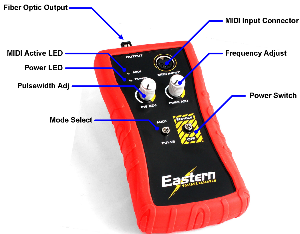
Figure 10 – Handheld MIDI Controller Functions / Connectors
